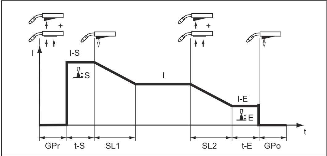
"Special 4-step mode" is particularly suitable for welding aluminium materials. The special slope of the welding current curve takes account of the high thermal conductivity of aluminium.
