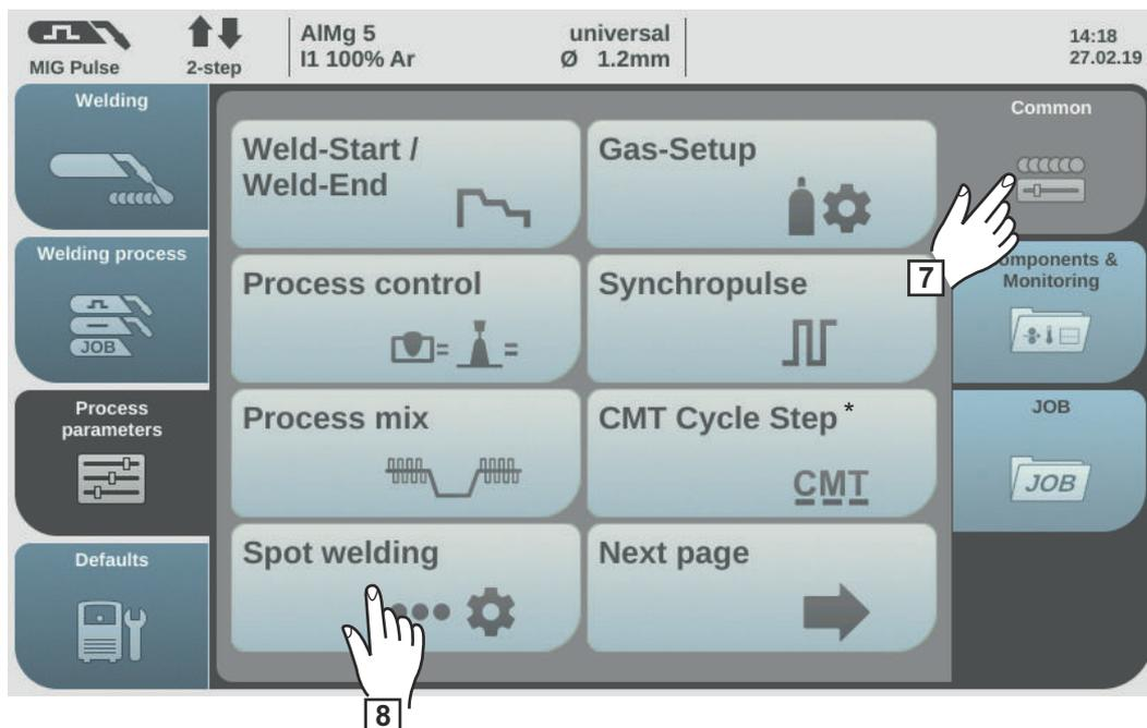
\* Only displayed if the OPT/i CMT Cycle Step option is present on the power source. In TWIN mode, the "TWIN process control" button is displayed after the "Process mix" button. In this case, the "Spot welding" button is on the next page.
