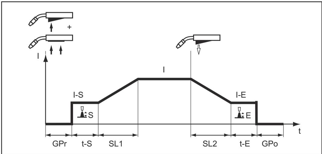
"Special 2-step mode" is ideal for welding in the higher power range. In special 2-step mode, the arc starts at a lower power, which makes it easier to stabilise.
