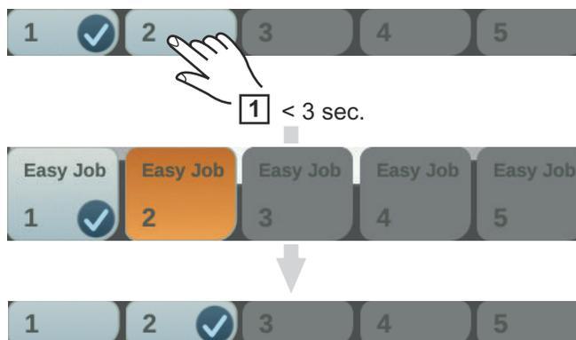
If a tick is not displayed after touching an EasyJob button, this means that there is no operating point saved under this button.
