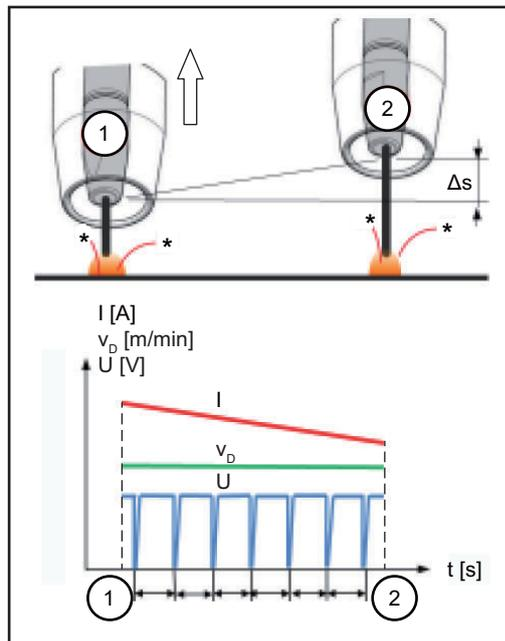
The advantages of a short arc are maintained even if the stick out is changed, since the short-circuit properties stay the same.
