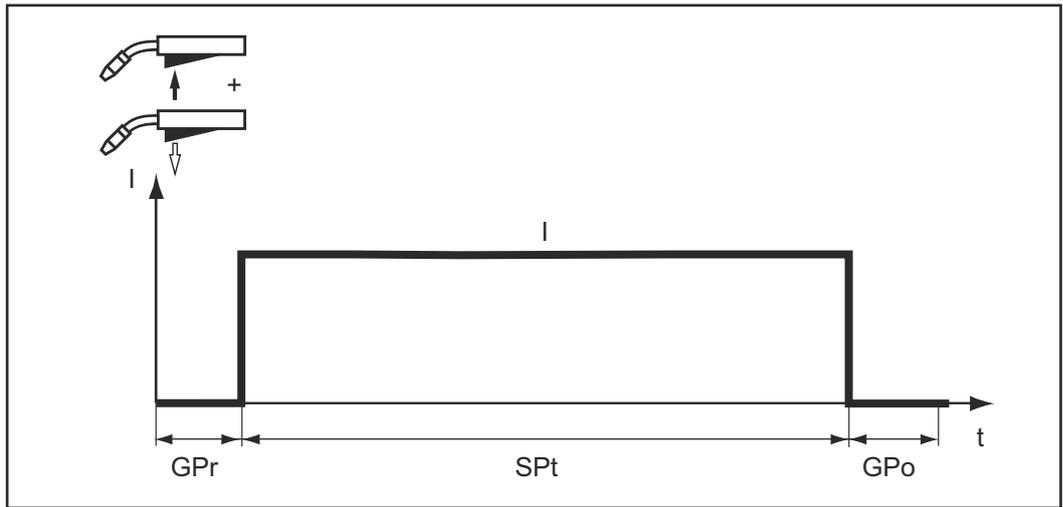
The "Spot welding" mode is suitable for welded joints on overlapped sheets.
