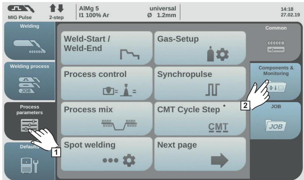
\* Only displayed if the OPT/i CMT Cycle Step option is present on the power source. In TWIN mode, the TWIN process control button is displayed after the "Process mix" button.
