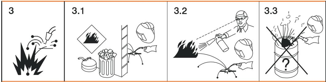
3 Welding sparks can cause an explosion or fire.
