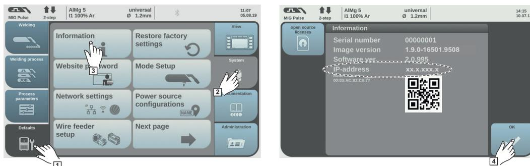
**1** Settings / System / Information ==> Note down the IP address for the power source
