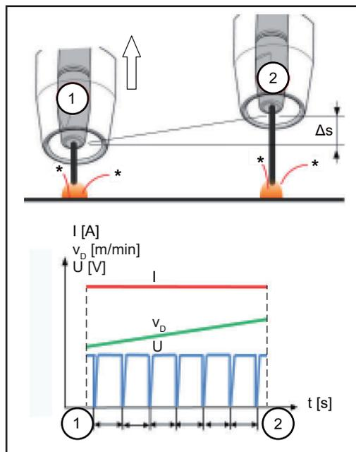
If the stick out is changed with the penetration stabilizer activated, the penetration also stays the same. The short circuit behaviour is controlled by the arc length stabilizer.
