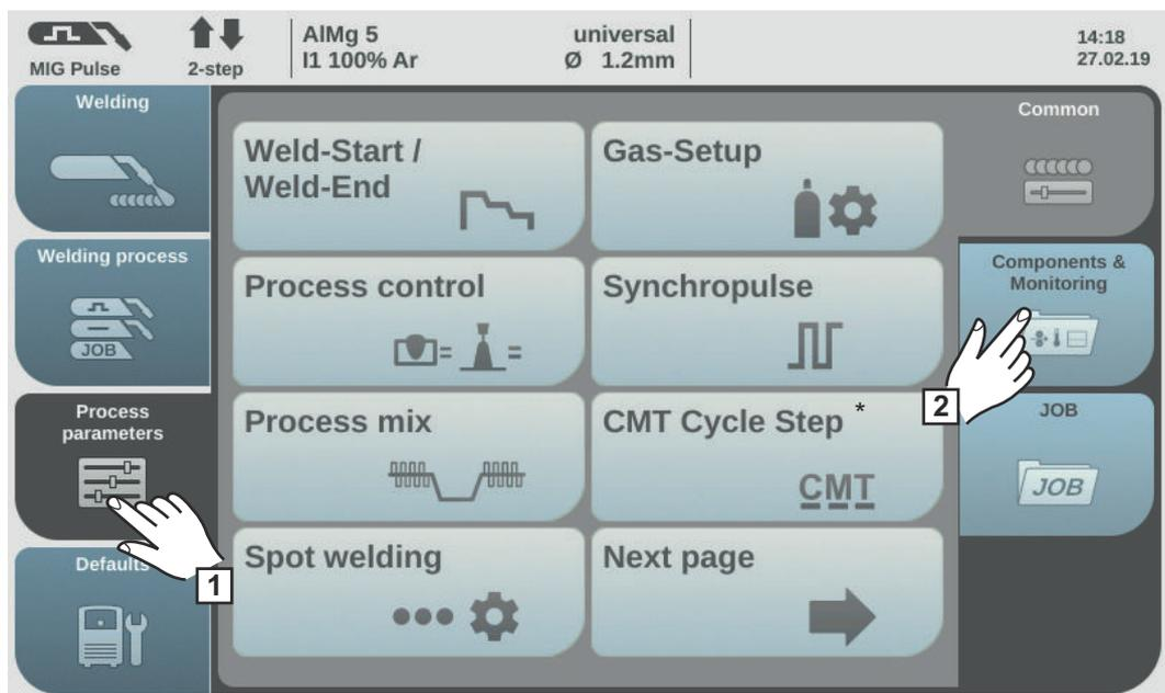
\* Only displayed if the OPT/i CMT Cycle Step option is present on the power source. If the system has a Twin robot interface, the TWIN Process Control button is displayed after the Process Mix button.
