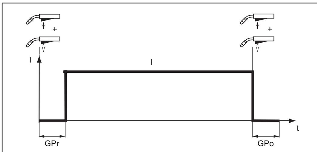
"4-step mode" is suitable for longer weld seams.
