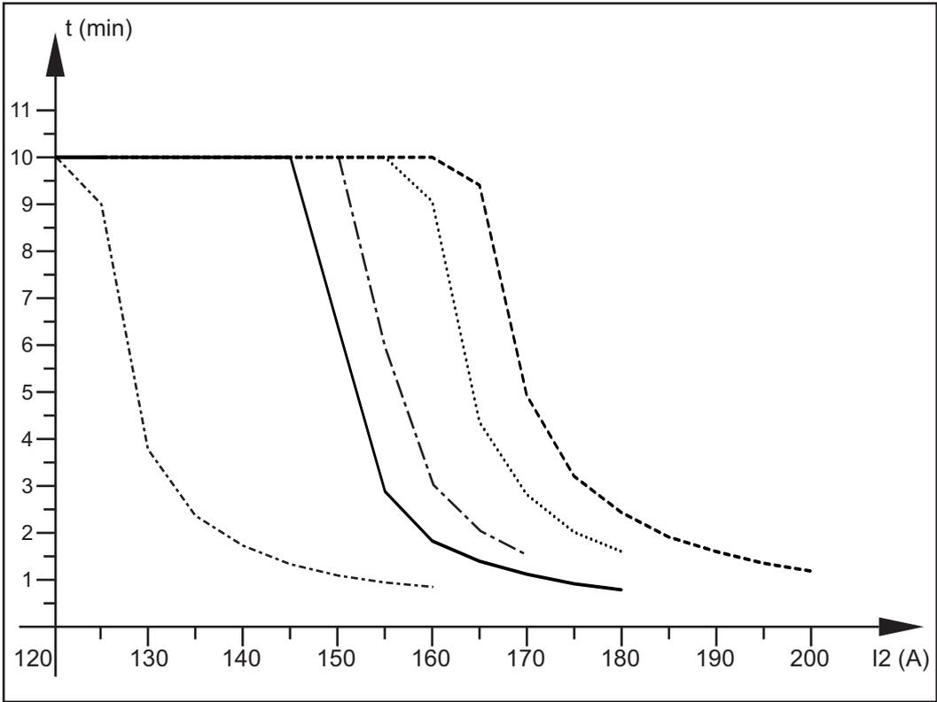
(1) Mains fuse protection 10 A (2) Mains fuse protection 13 A
