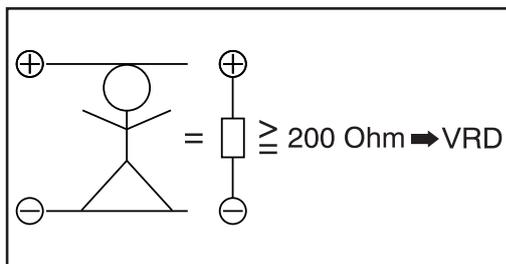
The welding circuit resistance is greater than the minimum human body resistance (greater than or equal to 200 Ohm):
