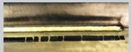
The Cromarod electrodes give excellent bead shape and self-detaching slag.
